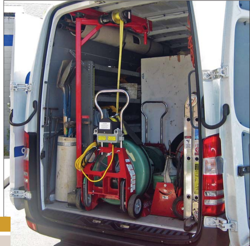
To prevent equipment damage and employee injuries, Frank Bonetti Plumbing of Castro Valley, Calif., has outfitted its service vans with the Vancrane, a rear-mounted, 1,500-pound-capacity electric crane made by Pickup Equipment Inc. (Photos courtesy of Frank Bonetti Plumbing)
